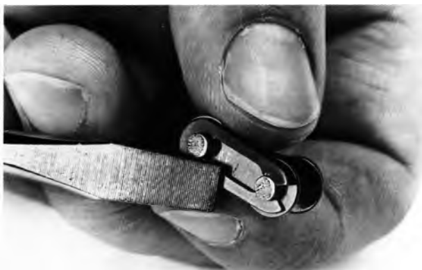
Coaster brake and three-speed bikes have chains that are connected at a master link, a special link that can be disassembled for removing the chain. There are two types. One is opened by flexing the chain and lifting off the sideplate; the other (see photo) is removed after prying off a spring clip.
