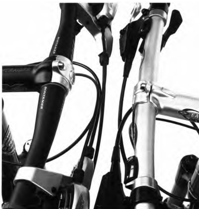
Handlebars and stems are available with various different clamp-surface diameters. Make sure you are certain of the size of your handlebar and stem before changing one or the other.
