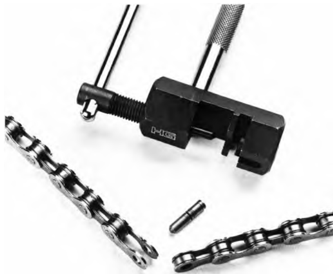
Chains are separated and put together with chain rivet or chain pin extractors (commonly known as chain tools).
