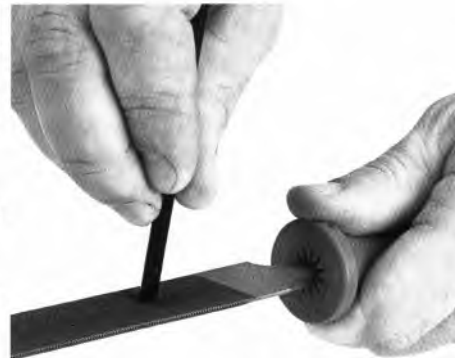
File the end of the housing flat so it doesn't try to bite-in under pressure and bind the cable.
