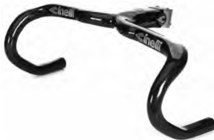
One-piece handlebar-and-stem combinations are incredibly lightweight, but they aren't as adjustable as individual components.
