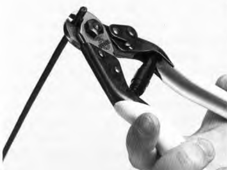
Cut cable housing using a sharp pair of cable- or diagonal-cutters.
