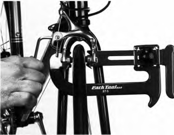
Use a third-hand tool to hold brake pads against the rim while the cable is being tightened.
