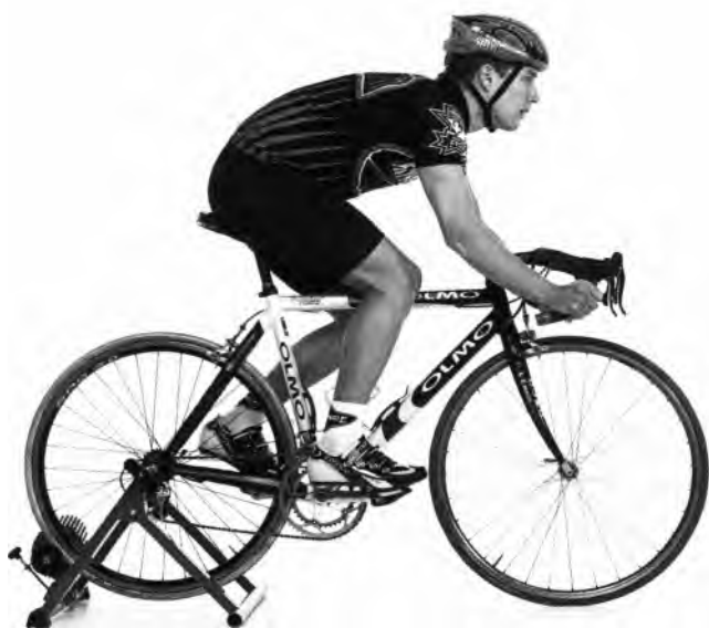
A dropped handlebar gives the rider a lower, more aerodynamic position on the bike.
