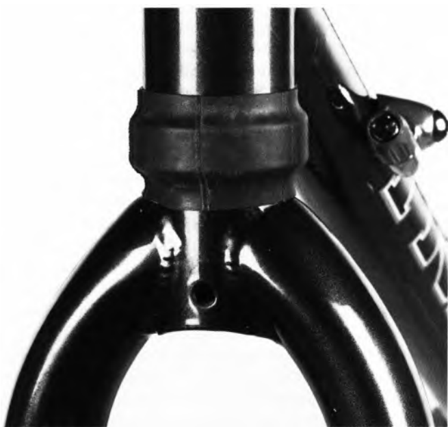
Fit short sections of an inner tube over the ends of the head tube during a headset overhaul, then pull them over the cups later to shield the bearings from wind and road grime.
