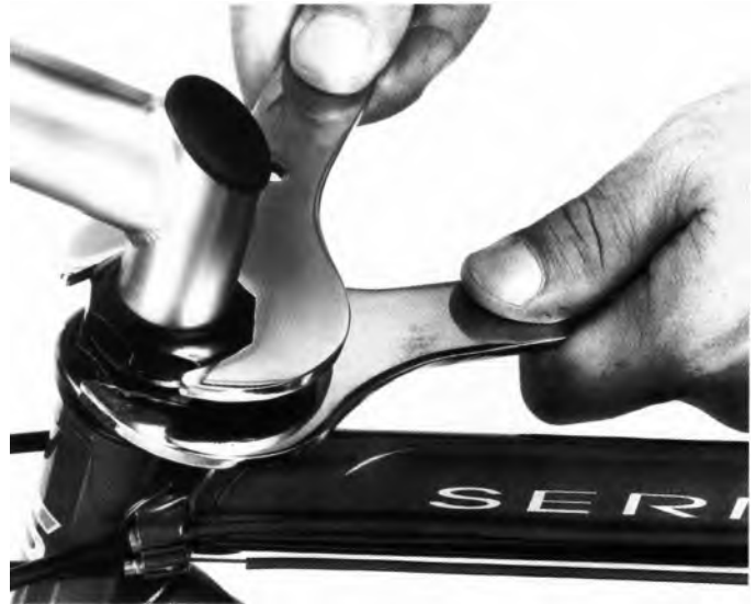
Use two headset spanners simultaneously to adjust a threaded headset: one on the locknut (top nut) and one on the adjustable cup (or cone).
