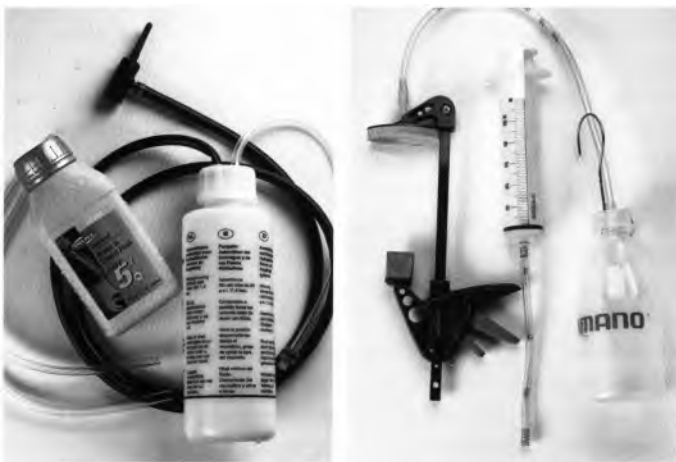
The basic principles of bleeding hydraulic disc brakes apply to all examples. Each manufacturer, however, has devised a system that it believes works best with that particular brake design. If you want to bleed your own brakes, it is highly recommended that you purchase a factory bleed kit tailored to your brake set and carefully follow the manufacturer's instructions.
