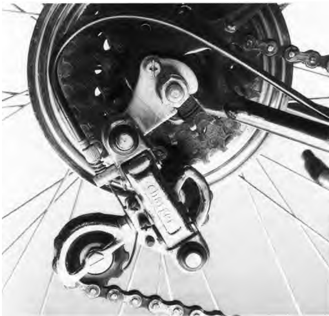
A less-expensive bike may feature a rear derailleur that is attached to the frame via a bolt-on hanger. It's a good idea to regularly check the nut that holds this hanger on the frame so it remains tight. Otherwise, the rear derailleur may come off when you remove the rear wheel, complicating reinstallation of the wheel.
