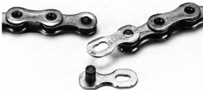
Certain derailleur chains have special connecting links (such as the SRAM Power Connector chain shown here) that make chain installation and removal easier because you can do it by hand.
